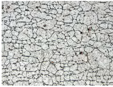
Fig. 6: Detail of Fig. 5. Note secondary grain boundary carbide precipitates, and primary titanium carbonitride precipitates (orange), 500x
