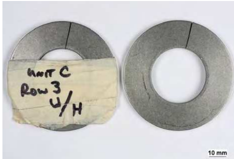
Fig. 2: Fractured disc springs in as-received condition
