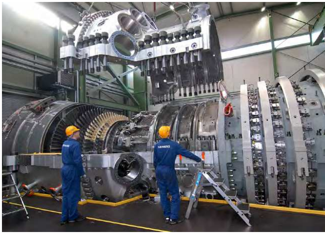
Fig. 1: Levers of variable inlet guide vanes of a gas turbine compressor (right) [Source: Siemens Media Database]
