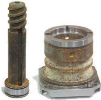
Figure 3.3 Rusted mold components
